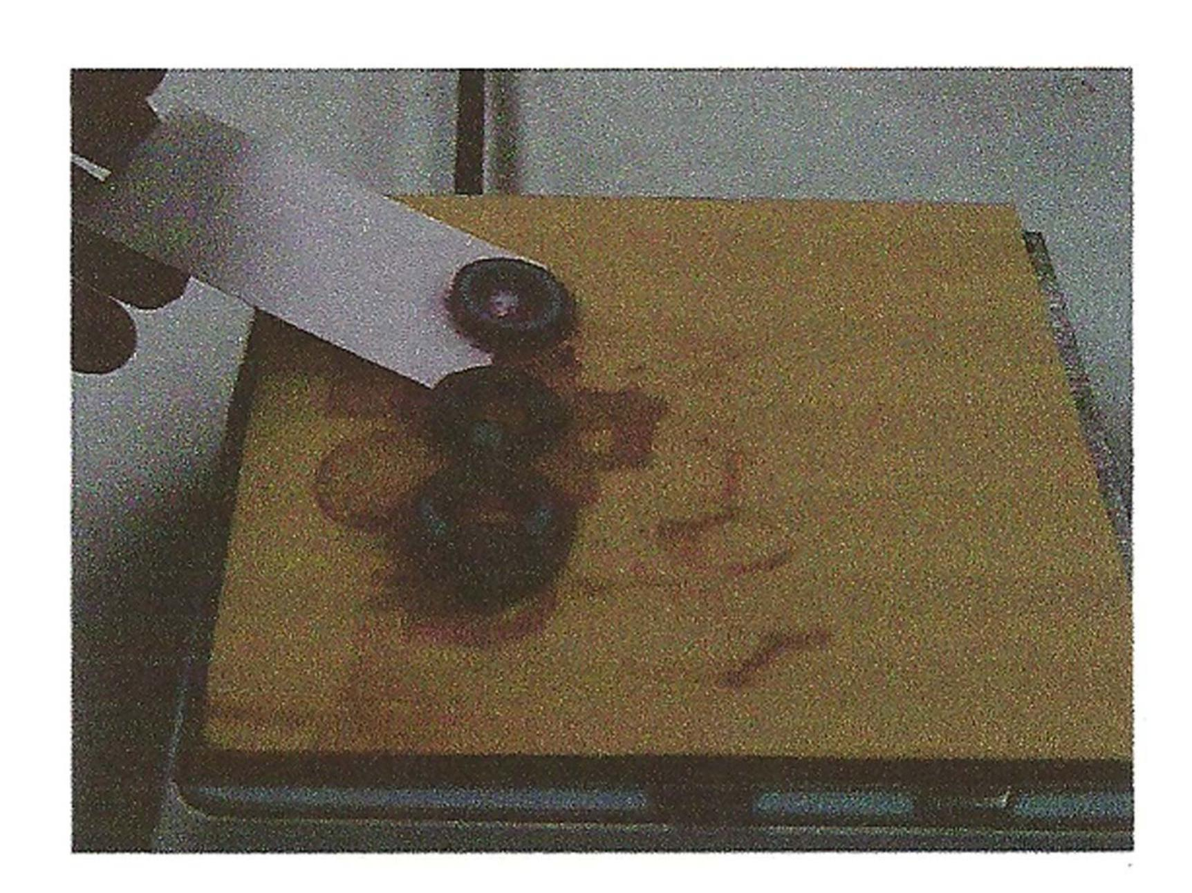
Once the InduraBase plate cools, it is ready for re-use on the unit. Selecting the Last Used Plate from the *Indurabase Setup* screen and then executing one foam cut will trim off any residual InduraFill left on the plate as a result of model removal.
