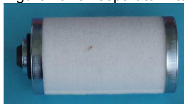
Figure 29: Oil separator filter of vacuum pump
