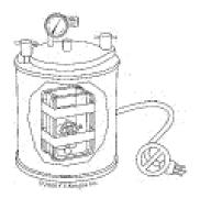
You can cure the mold inside your empty and unheated air-pressue type wax injector, using the pressure to collapse air bubbles rather than a vacuum to remove them.
