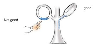
Do not place waxes/plastic parts to close to flask cylinder. There should be a distance of at least 5 mm.
