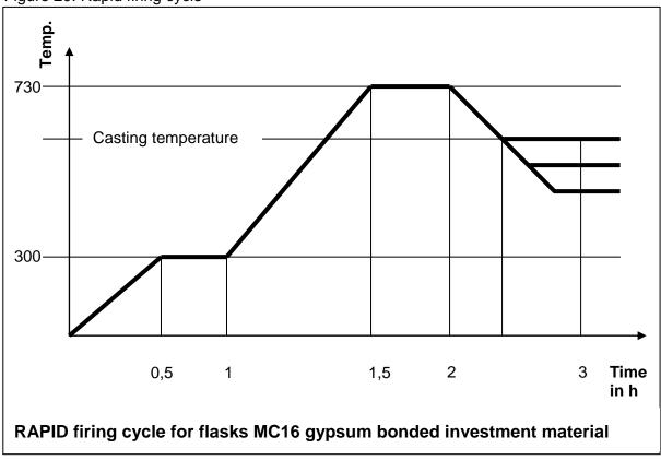
**Caution:** In case of a "gentle"-firing cycle all amenities of the investment material are prevented from damage. A rapid firing cycle doesn't take care on these amenities. Already aged investment powder or thus of lower quality can react because of gruff handling with cracks.
