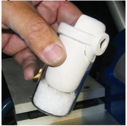
Place crucible with glass inductor shield in the induction coil.
