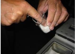
The crucible should be sitting easily on the quartz fleece. The crucible collar should be close to the glass inductor shield.
