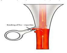
Liquid metal is heavy; it can break away thin parts of the gypsum. Create all connections in hydrodynamic proper style
