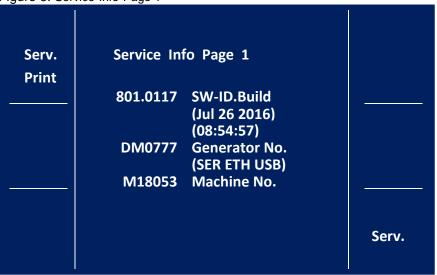
If you press "Serv."-button again, you'll see cooling water flow (sensor 0), generator temperature (IGBT) and actual machine state. The rows 'Water flow 1' and 'Op.' are not used in MC16. The button 'Serv. (Service) Print' is without function.
