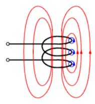
If now a conductive material like metal is brought into this induction field, metal absorbs energy, it couples. This metal is separated in a nonconductive ceramic crucible in between.
