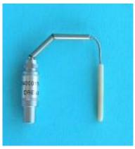
Important: Use thermocouple for melting only in crucibles with graphite inlet. Otherwise induction energy will stimulate thermocouple directly (without protection by graphite). Result, read in display, is pure nonsense!
