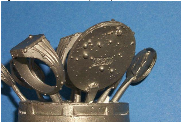
Figure 24: bubbles - incomplete spheres
