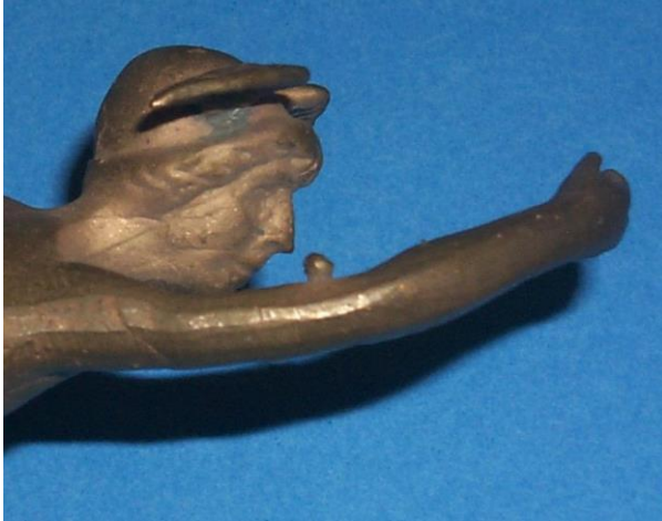
Figure 23: bubbles - complete spheres
