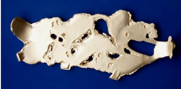
Figure 21: horizontal flashing or finning
