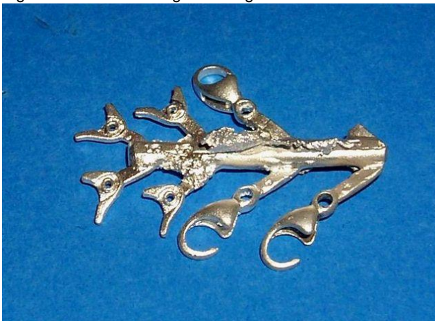
Figure 22: other flashing or finning
