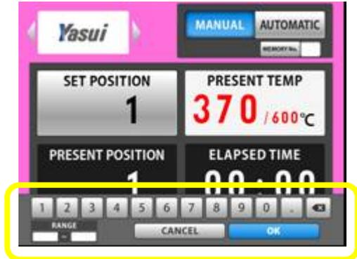
2) Rotation will stop at the point you've entered. The present back ground color will turn green. This is to prevent leaving rotation suspended. Do not forget to push rotation button for 2 seconds after taking flask out of furnace.
