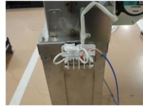
12) Install Afterburner on RBF
