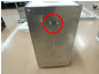
insert thermocouple in place.
