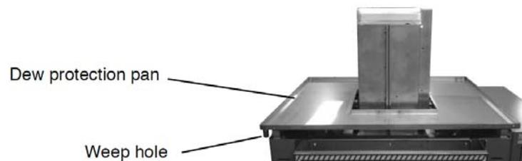
14) Place afterburner fan unit with adiabatic and dew protection plate on Afterburner body, and fix it by bolts using a hex key.
