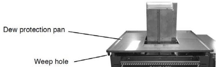
14) Place afterburner fan unit with adiabatic and dew protection plate on Afterburner body, and fix it by bolts using a hex key.
