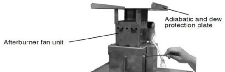
15) Connect cables for afterburner fan by pushing connectors together.
