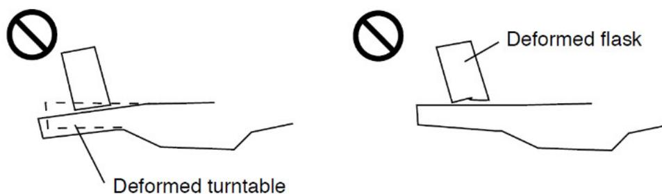
(The turntables are used in high temperature environments, so their deterioration speed depends on individual using frequency and conditions.)
