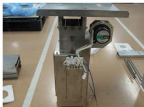
Connect the cables for sheath heater and thermocouple to the area marked by red circle. At this time, take care that the polarities of the thermocouple must match.
