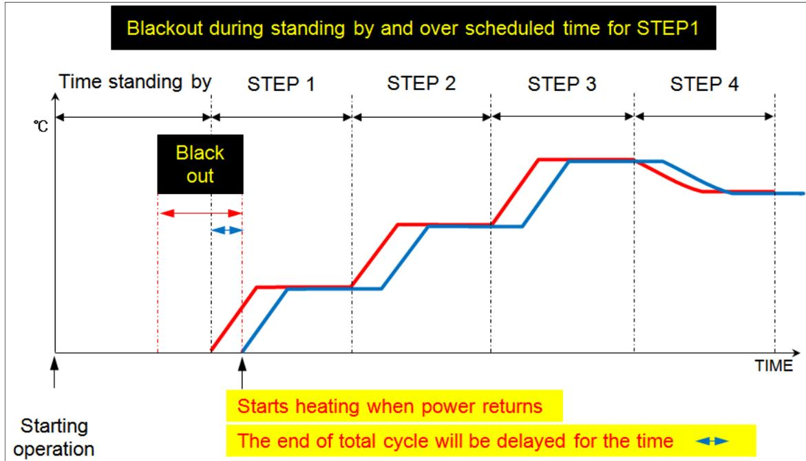
4) AUTOMATIC BURNOUT MODE (during burnout cycle time within 5 minutes)
