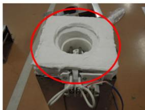
Place the adiabatic bracket for fan on the area marked by red circle and install the fan.
