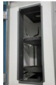
7. Always keep clean inside of the furnace. Investment residue or dusts on the turntable or the wax drain unit may cause clogging and prevent wax from draining out of the furnace.
