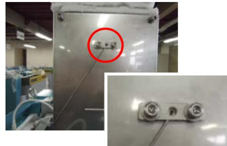
7) Place afterburner unit to fit at central hole on top of furnace, and fix it with four bolts removed by the former procedure 4).
