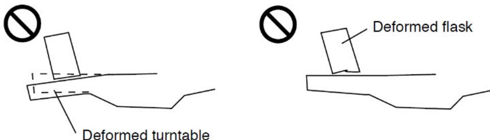
(The turntables are used in high temperature environments, so their deterioration speed depends on individual using frequency and conditions.)
