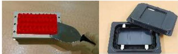
\* Do not expose the resin tank to direct light source because the resin will solidify under UV light. Use tray to cover the resin tank to prevent solidify.
