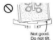
3) Slide the mold chamber in and out for trial to check that the flask automatically moves up and down.
