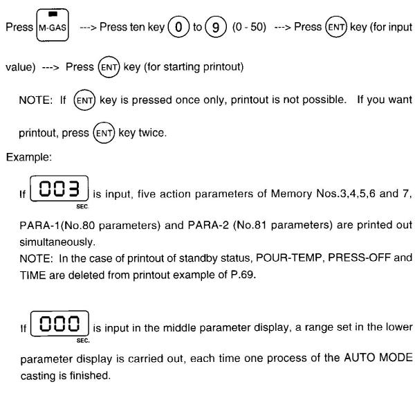
3) Printout range is set by input of value in the lower parameter display. ---maximum 3
