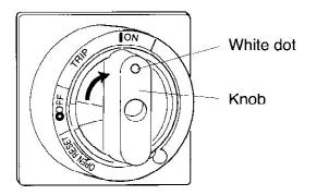
IMPORTANT: When the white dot of the BREAKER switch moved to TRIPPED position during use of the machine, overcurrent has flown inside the machine (the machine became TRIPPED condition by overcurrent). In this case, check the cause and take necessary action. Then, turn the knob to RESET position. Next, turn the knob to ON.
