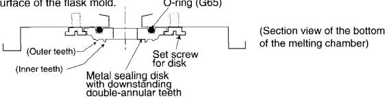
IMPORTANT: Wrong fixation of the metal sealing disk with downstanding double-annular teeth may greatly affect casting results. Check the below [1] to [4].
