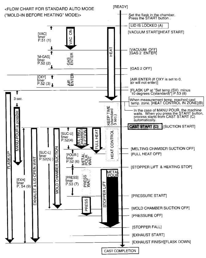
In the case of MANUAL POUR mode, you have to press the START button once again to activate **CAST START (C)**.
