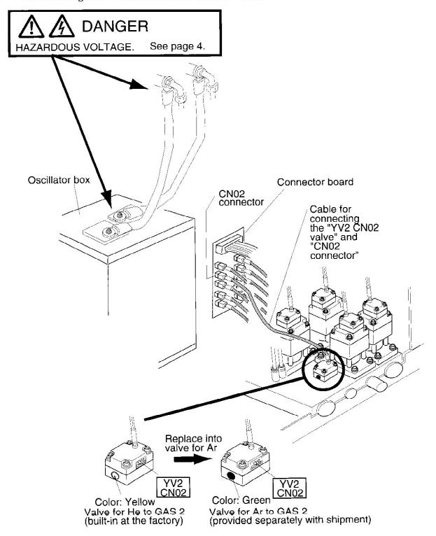
3) Remove the four nuts at the bottom of the valve for Ar to GAS 2.
