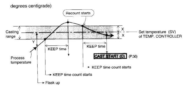
When measured present temperature goes out of the Casting Zone during the KEEP time, counting of time starts again when temperature again enters into the Casting Zone.
