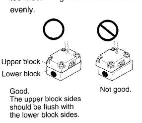
Valve for Ar Green Adjust the position of valve so that position of ports should coincide each other. 5) Taking care of the direction Threaded holes (x 4) for "YV2 CN02 valve" of the connector, push in the connector of connecting Connector board cable to the connector board as the figure. Connect to the CN02 connector (located at left side and second from top on the connector board) Valve for Ar to GAS 2 (provided separately with shipment) Green
