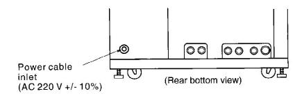
Gasket for power cord of the machine (Fix the electric cord with the gasket.)
