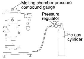
At this time, watching the needle movement of display value of melting chamber pressure compound gauge, adjust the pressure regulator of the gas cylinder, so that time period from vacuum (about -0.1 Mpa) to atmospheric pressure (0) should be within about 10 to 12 seconds.
