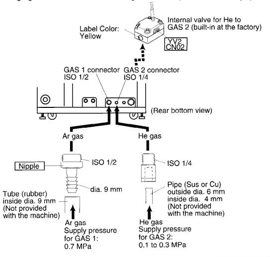
IMPORTANT: He gas pressure has an effect on gas substitution level. Therefore, set He gas pressure at same value every day. To make fine adjustments of He gas pressure, activate the machine and check actual gas injection speed as follows:
