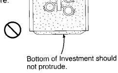
Remove a lump of investment powder residue from this area if there remains any, so that the flask will not tilt when it is set in position. /
