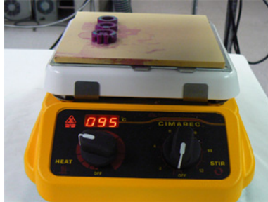
Figure 11-2 Heater Stirrer with build plate
