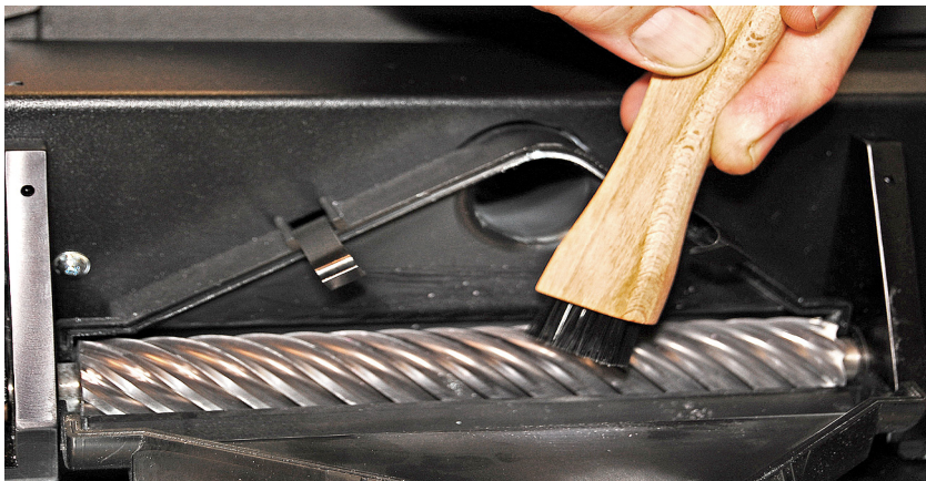
Figure 3-6 Cleaning the Cutter Blade
