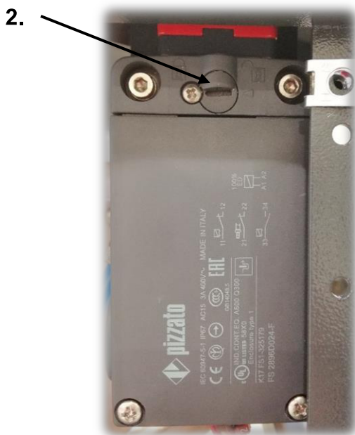
Fig. 2.19 Safety device to lock the lid
