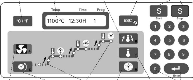
Air Control (available on air exchange models only) activates the air exchange feature for a chosen stage during a firing cycle. Press once for S1 (stage 1), twice for S2 (stage 2) and three times for S3 (stage 3). Press ENTER to stage new value. A setting of 0 means fan is off. A setting of 9 means maximum air exchange.
