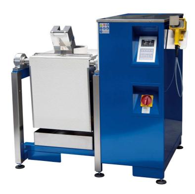
This modern melting furnace has been designed to melt fast and safe large amounts of gold, silver, brass, bronze and aluminum alloys. Due to the strong induction generator the melt will be mixed homogenous. The tilting process can be carefully controlled by a joy stick. All relevant data are shown on the integrated LCD display. The standard **GSM-modem** guarantees easy maintenance and service.
