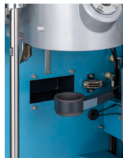
Graphite protection pot for metal leakage
