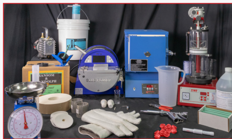
After pouring, the MC series automatically switches to overpressure to optimize the cast, designed specifically for delicate and fillgree parts.
