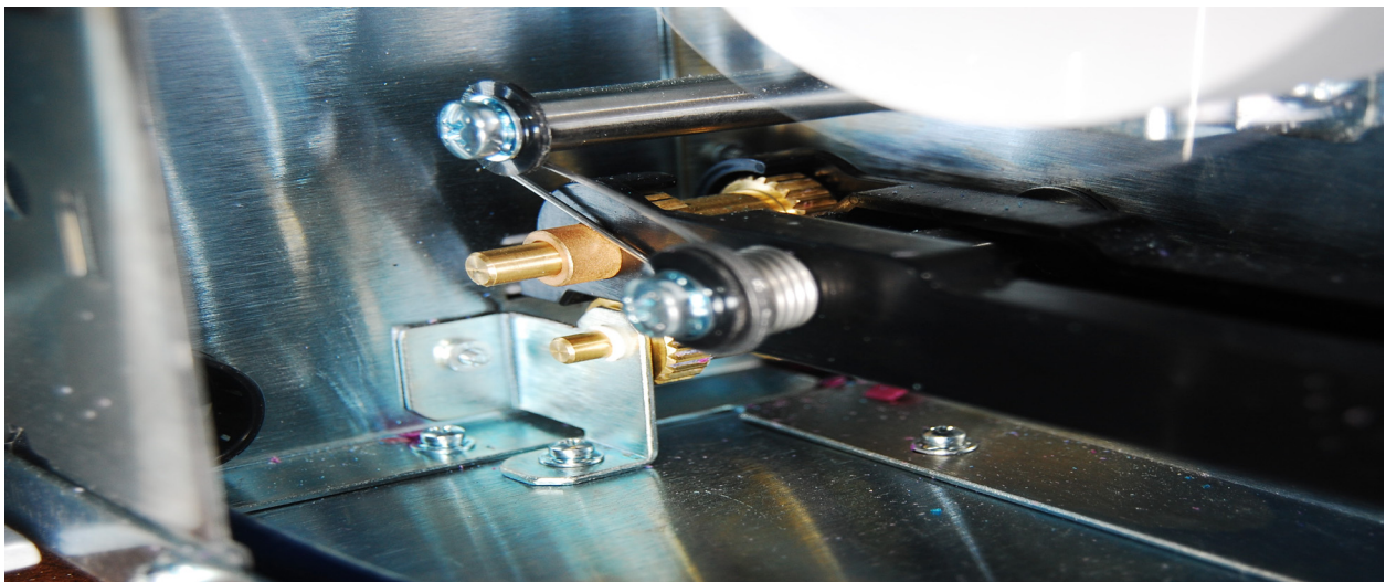
Figure 7-9 Cleaning the Paper Tape Feed Assembly
