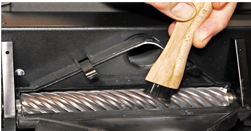
Figure 3-6 Cleaning the Cutter Blade
