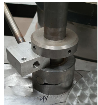
Figure 1 showing block used to lift the mixing chamber up
