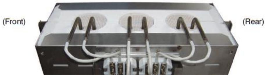
6) Insert the tip of thermocouple tube into the hole for thermocouple as below figures.
