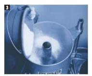
**3.** The weighed investment material is filled into the stirring container. The mixer is sealed with a plexiglass lid which allows surveillance of all procedures. Now the investment material is mixed with the water under vacuum. Through the opening of the filling taps the underneath placed flasks are filled while still under vacuum. This procedure and simultaneous vibration allows flasks of highest quality to be produced.
