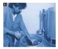
**1.** 3 flasks are placed in the mixer and the stirring unit is swivelled over them.
