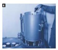
**4.** To clean the machine the mixer is swivelled over the drain bowl and then cleaned with a spray nozzle.
