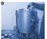
**4.** To clean the machine the mixer is swivelled over the drain bowl and then cleaned with a spray nozzle. The stirring unit is hereby raised by 100 mm using a compressed-air cylinder.
