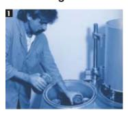
**1.** 8 flasks are placed in the mixer and the stirring unit is swivelled over them.
