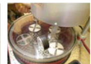
Mixed slurry poured via valve to each flask in turn, with aid of turntable
