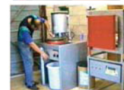
Mixed slurry poured via valve to each flask in turn, with aid of turntable
